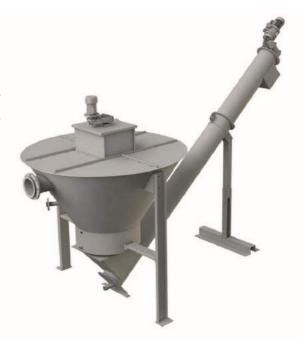
The washed sands are removed from the bottom of the hopper by a shafted screw conveyor, while the output cleaned water outflows from a pipe placed at the top of the hopper.
