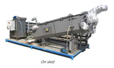
To obtain the best performance in terms of sludge dewatering, the two machines can be installed one after the other: first the thickener to obtain a concentration, variable depending on the model from 4 to 8% of SS, and to follow the dewater screw press for dewatering, with a dry matter percentage up to 25%. The dewatering screw press is particularly suitable to thicken and also dehydrate the material from flotation units.
