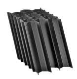
Lamella clarifier or also known as inclined plate separator is designed to remove particulates & sediments from liquids. They serve as primary and tertiary clarification system for sewage or industrial waste streams. It provides a large effective settling area, resulted up to 80% less footprint compared to a traditional settling tank.
