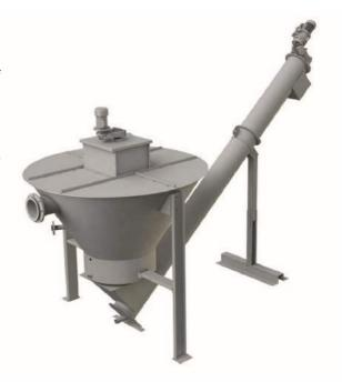
The washed sands are removed from the bottom of the hopper by a shafted screw conveyor, while the output cleaned water outflows from a pipe placed at the top of the hopper.
