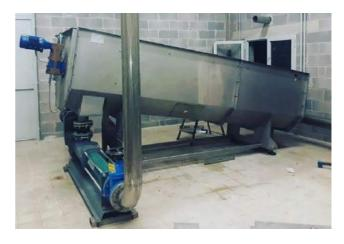
After reaching the discharge zone, the sludge is conveyed towards the outlet, situated on the bottom of the machine which in the case of the thickener can be connected to a pump which transfers the product to a possible subsequent dehydration system, while in the dewater screw press, once passed the pneumatic counter pressure system, the sludge is discharged within special dumpster or is loaded into a transport system made with screw conveyors or with transport belts.
